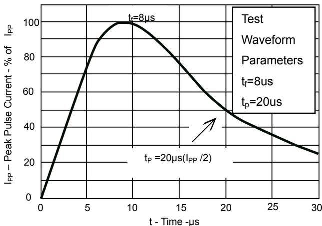
Fig 1. Pulse Waveform
